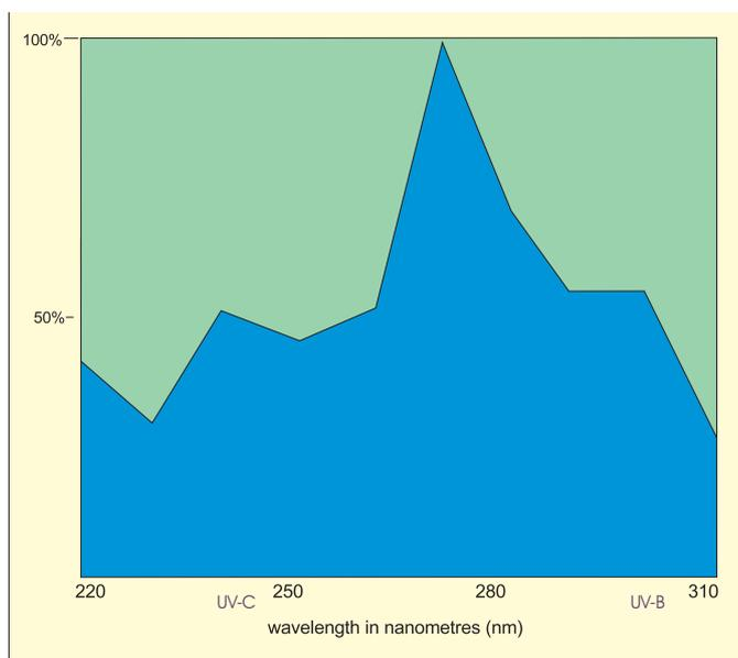
Figure 3 Relative sensitivity of the human cornea to UVC and UVB, (reciprocal of threshold energy for damage) after Pitts (1974)
