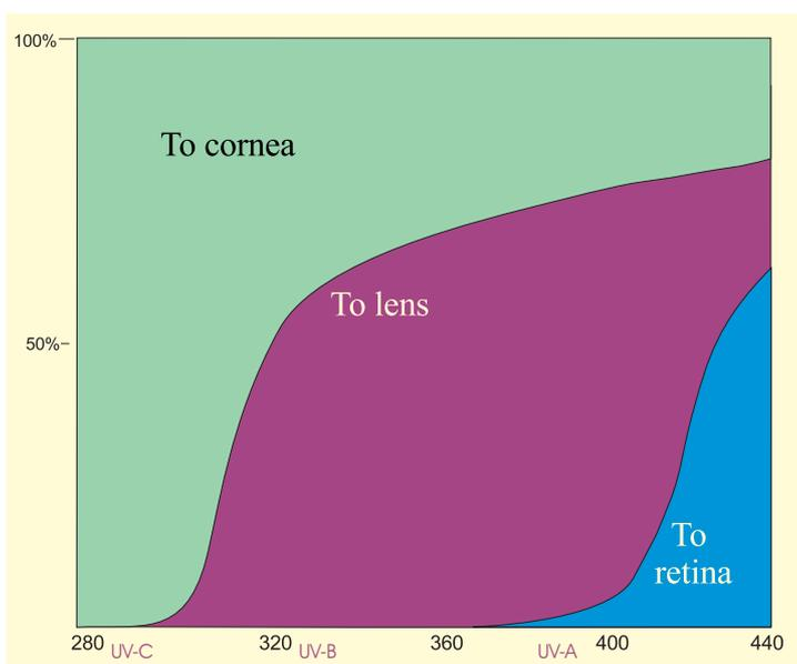
Figure 4 Transmittance of near UV to the lens and retina after Charman (1990)
